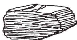
Easily split layers of 0.0001-cm-diameter particles cemented together
