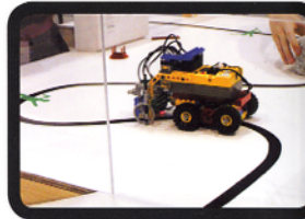
Some robots use light sensors to follow a visible trail.
