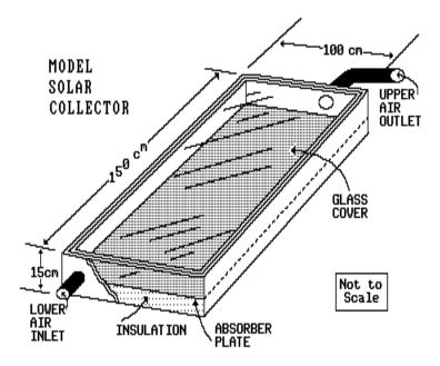
The solar collector is placed outside in sunlight, facing south and tilted 40° from the horizontal. At which position of the Sun would the collector receive the most intense solar radiation?
